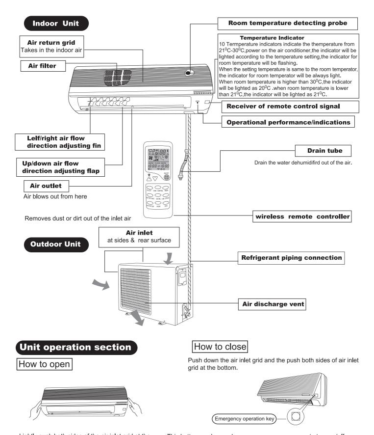
Lightly push both sides of the air inlet grid at the botton and pull it to this side till a resistance is felt.
